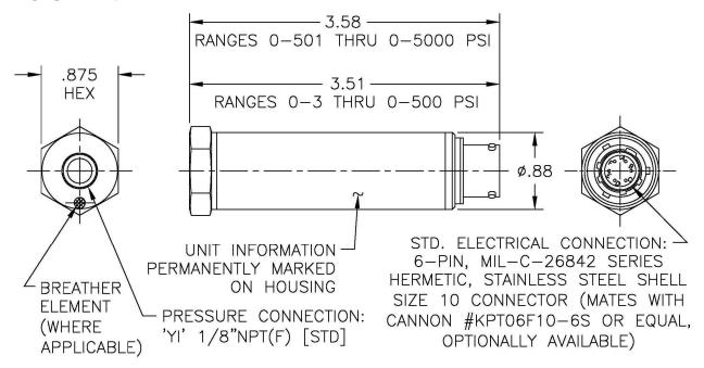
**Excitation Voltage:** 9-30 VDC; 12-30 VDC for 5 < output < -5 VDC
