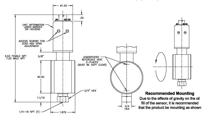
MODEL 244 MODEL 344 Connector: Connector: PT02E-10-6P PT02E-10-6P Input: Input: 10 - 42 VDC 10 - 42 VDC **Output: Output:** 0 - 5 VDC 4-20 mA **Cal Shunt: Cal Shunt: 80% FSPR** 80% FSPR
