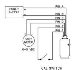
Viatran recommends grounding the case of the unit to avoid instability of the output signal.
