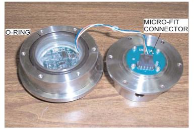
From the replacement kit remove the replacement sensor 'O'-Ring & package of grease. Grease the 'O'-Ring and place it in the groove. Attach the Micro-fit connector to PC board on the new adapter.
