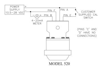
To activate cal on Model 520, the cal circuit must be powered.Input:10.5 - 28 VDCOutput:4 to 20 mACal Input:7.0 to 28 VDC
