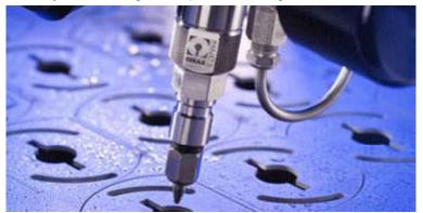
at high velocity and pressure, or a mixture of water and an abrasive substance. The process erodes the materials in the same way as water erosion found in nature but accelerated and concentrated through high pressure. It is often used in the fabrication or manufacture of parts for machinery and other industries. It is used in applications in the mining to aerospace industries where it performs operations such as cutting, shaping, carving, and reaming.
