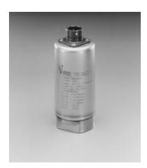
The "46" Series measures pressures over the standard range of 25" HgA to 32" HgA. Model 246 provides a 0-5 VDC output signal, while the Model 346 offers a 4-20 mA signal. Both barometers have infinite resolution, an operating range of -40° F to 250° F, and readily accessible external zero and span adjustments. There are also numerous pressure ports and electrical connections available to suit specific application needs.
