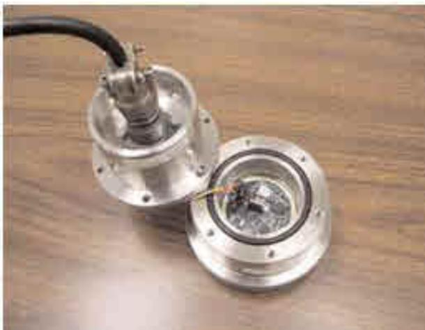
Insert the 5-pin serial connector cable as shown below. The white mark on the cable must be positioned closest to the outer edge of the PC board for proper operation.
