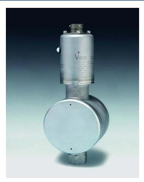
The Model 244 provides a 0 to 5 VDC signal, while the Model 344 offers a 4 to 20 mA signal. Using our variable capacitance technology, the 244 and 344 transducers provide extreme overpressure protection up to 500 PSI.
