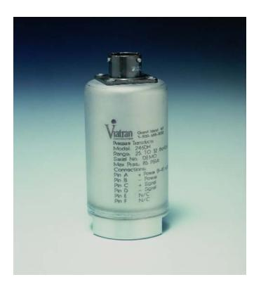
The X46 Series measure pressures over standard ranges of 25" HgA to 32" HgA. Model 246 provides a 0-5 VDC output signal, while the Model 346 offers a 4-20 mA signal. Optional Full Scale Pressure Ranges (FSPR) and output signals are available.
