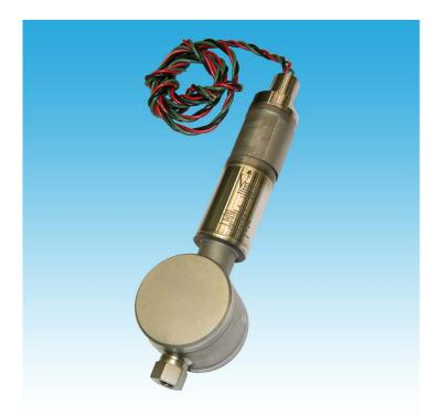
Viatran's Model 544 is a gage pressure transmitter designed for precise measurement in harsh environments. Its all welded 316 stainless steel construction ensures durability and corrosion resistance, and it offers overpressure protection to 500 PSI.
