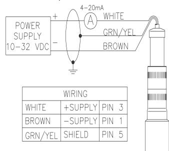
The 595 detachable level transmitter can be powered by a DC power supply ranging from 10 to 32 volts. See installation manual for more details.
