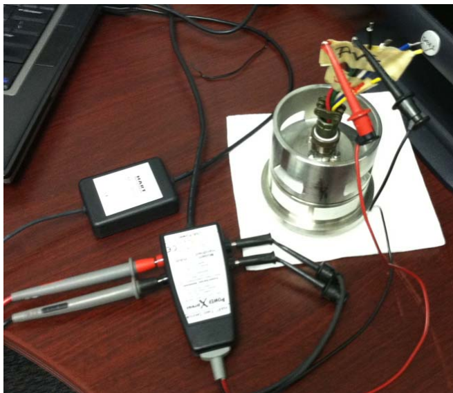
Figure 4 Example of a set up using the PowerXpress HARTTRIM Rev. B
