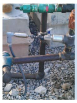
Measurements for casing and tubing pressures
