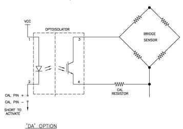
NOTE: Isolated, internal shunt calibration (6 pin connector required).
