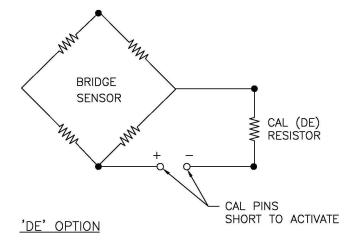
NOTE: Internal shunt calibration.
