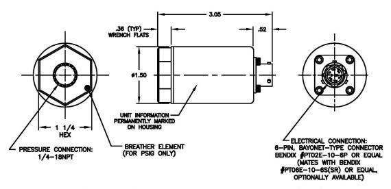
**Sensor Construction and Wetted Materials:** Solid Machined Diaphragm: 15-5PH Stainless Steel
