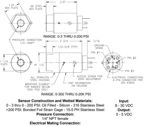
4-Pin, DIN 43650 box mount connector
