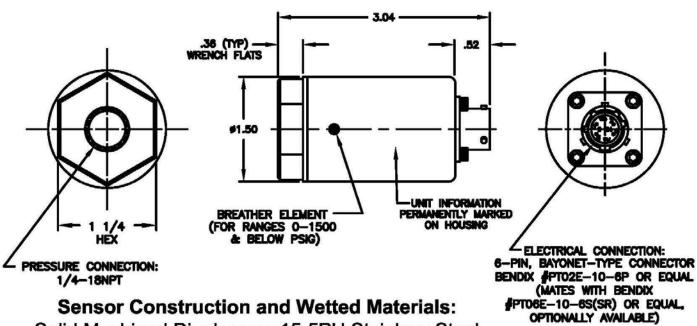
Solid Machined Diaphragm: 15-5PH Stainless Steel
