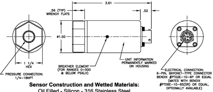
Oil Filled - Silicon - 316 Stainless Steel Pressure Connection:
