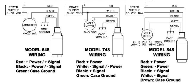
Note: If the unit is certified for hazardous locations as Intrinsically Safe, use the enclosed connection diagram. Only the pressure transmitter is considered to have the Factory Mutual, CSA or ATEX safety ratings. If you have purchased a transmitter and isolator/remote seal, they have not been tested as a system for safety certification. The end-user shall be responsible for verifying the system is safe and installed accordingly.
