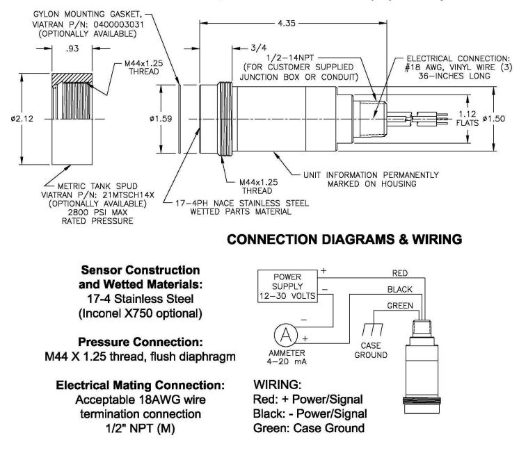
Note: If the unit is certified for hazardous locations as Intrinsically Safe, use the enclosed connection diagram. Only the pressure transmitter is considered to have the Factory Mutual safety ratings. If you have puchased a transmitter and isolator/remote seal, they have not been tested as a system for safety certification. The end-user shall be responsible for verifying the system is safe and installed accordingly.
