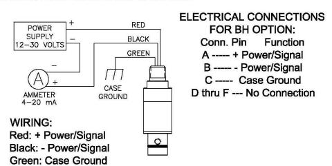
Note: If the unit is certified for hazardous locations as Intrinsically Safe, use the enclosed connection diagram. Only the pressure transmitter is considered to have the Factory Mutual safety ratings. If you have puchased a transmitter and isolator/remote seal, they have not been tested as a system for safety certification. The end-user shall be responsible for verifying the system is safe and installed accordingly.
