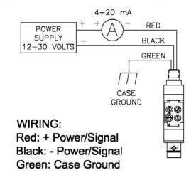
Note: If the unit is certified for hazardous locations as Intrinsically Safe, use the enclosed connection diagram. Only the pressure transmitter is considered to have the Factory Mutual safety ratings. If you have puchased a transmitter and isolator/remote seal, they have not been tested as a system for safety certification. The end-user shall be responsible for verifying the system is safe and installed accordingly.
