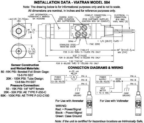
lote: If the unit is certified for hazardous locations as Intrinsically Safe use the enclosed connection diagram.
