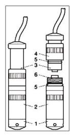
NOTE: Do not twist the sensor head when attaching it to the cable section!
