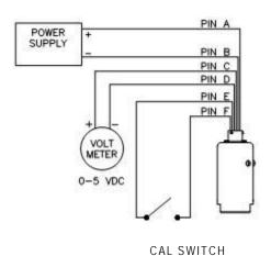
For best noise immunity, Viatran recommends connecting the shield of the cable to the housing and grounding the housing.
